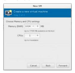
8. For the memory and CPU settings, specify values that match your system. For the purposes of this procedure, the values 4 GB RAM (4096 MB) and 4 CPUs are specified. Click **Forward**.
